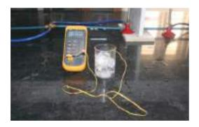
**Demonstration 7:** Measure mV developed in a thermocouple with a spirit lamp; 30 to 32 mV. Means about 750°C to 800°C; the same sensor can also measure 1200°C to 1400°C.
