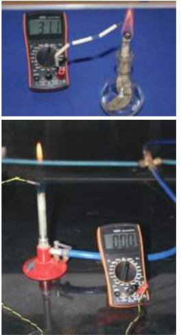
**Demonstration 8:** R vs T of  $Pt_{100}$ in ice and flame, then  $Pt_{100}$  digital thermometer. Time taken so far: 45 Min.
