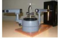
**38. Newton's Rings** In this experiment, we determine the radius of curvature of a given convex lens using Newton's rings experiment. The travelling microscope is moved slowly to the one side to cover, say, twenty-one dark rings. The rings are counted as n, n+3, n+6 up to n+21. The vertical cross wire is made tangent to  $(n+21)^{th}$  dark ring and the reading in horizontal scale is noted.
