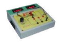
3. To study full and half wave rectifier circuits Draw the waveform of a half wave and full wave rectifier circuit and compare the Output VDC by using the multimeter. We observe a half wave and full wave rectifier output through CRO.
