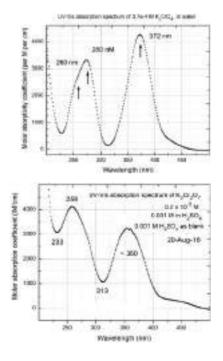
98. Complementary colours – Correlation of absorption spectra to colours If a compound absorbs green light, the compound appears red to our eyes. This is verified in this experiment.
