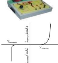
48. Light emitting diode (LED) characteristics\* We find the voltage for different colour LEDs. From this experiment we verify the  $E = h\nu$  (J). For Red LED 1.9 eV, for green LED 2.1 eV, green LED 2.2 eV and for blue LED 2.8 eV.
