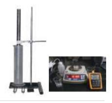
$$\alpha = \frac{\Delta l}{LX(T_2 - T_1)} \circ C^{-1}$$
