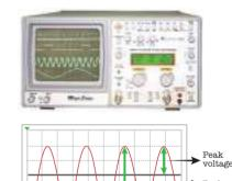
2. Diode Characteristics/ LED/Zener diode In this experiment, we draw the forward and reverse bias characteristics curve of a semiconductor diode. And determine knee voltage and bulk resistance.
