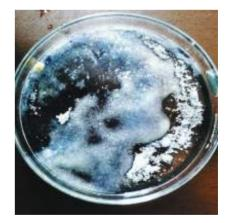
27. Double displacement reactions When solutions of sodium sulphate and barium chloride are mixed, a double displacement reaction occurs. One of the products, barium sulphate precipitates out since it is insoluble in water.
