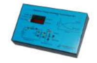
7. Current and Voltage phase difference in RC circuit\* In an AC circuit containing resistor (R) and capacitor (C), the voltage across the resistor is in same phase with current and the voltage across the capacitor lags behind the current by 90°. Use CRO to find this. From the figure we can find phase difference by using
